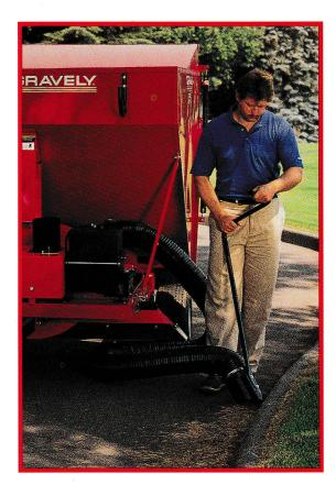
The 1050 features an optional  $6" \times 10"$  hand intake hose that can greatly reduce labor time by vacuuming material from flower beds, under shrubs, along fence lines and around markers or trees.
